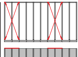
3. A minimum of 1 cross bracing must be fitted to each third double bay to stabilize the shelving system. Made from galvanized sheet steel. The stiffening diagonals, made of galvanised plate, are not necessary for shelving units 1010 mm high.
