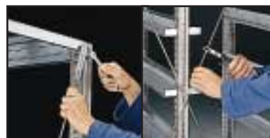
3. A minimum of 1 cross bracing must be fitted to each third double bay to stabilize the shelving system. Made from galvanized sheet steel. The stiffening diagonals, made of galvanised plate, are not necessary for shelving units 1010 mm high.
